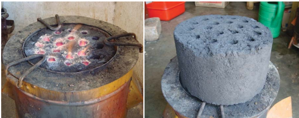
Above: left: An energy cooking stove; Right: A briquette made out of bio-waste. Pictures courtesy Nature Palace.
